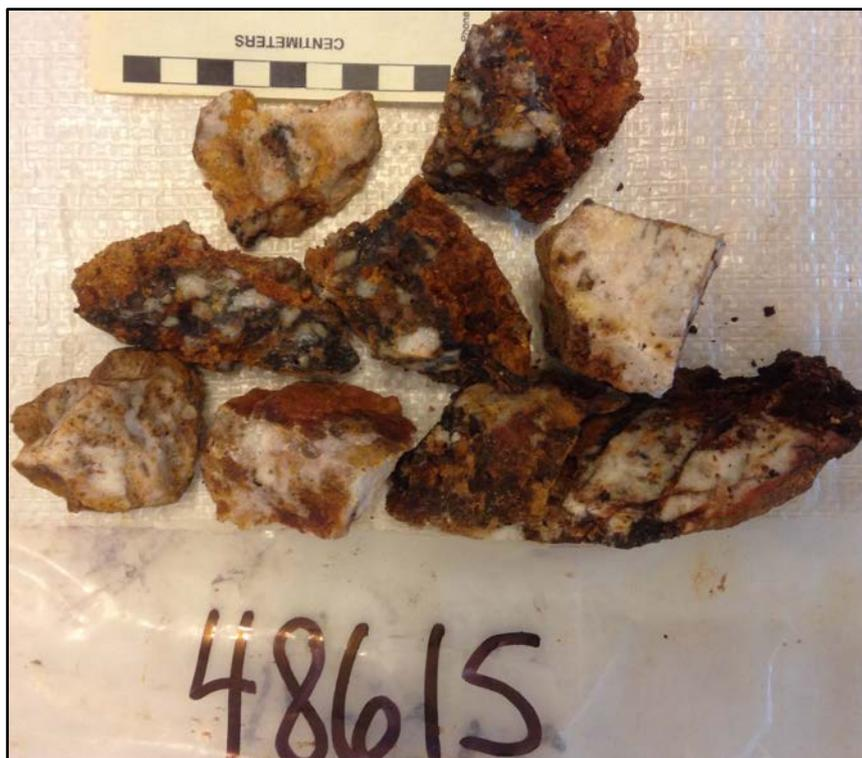
Figure 4 Topacio NE vein – Sample from artisanal ore pile (52.4 g/t Au and 158g/t Ag)
