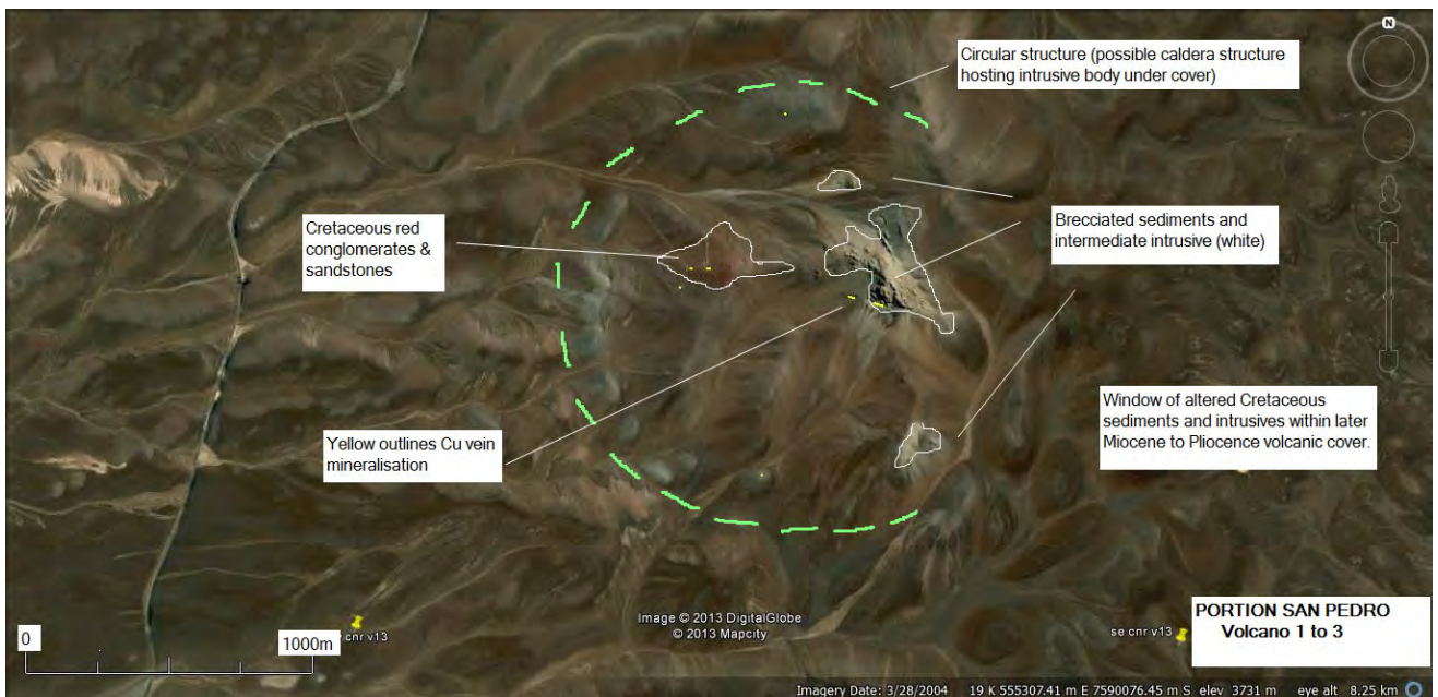
Figure 4. Satellite Imagery San Pedro Project. Inlier of Cretaceous sediment showing alteration associated with intrusive activity into sediments in possible caldera structure.
